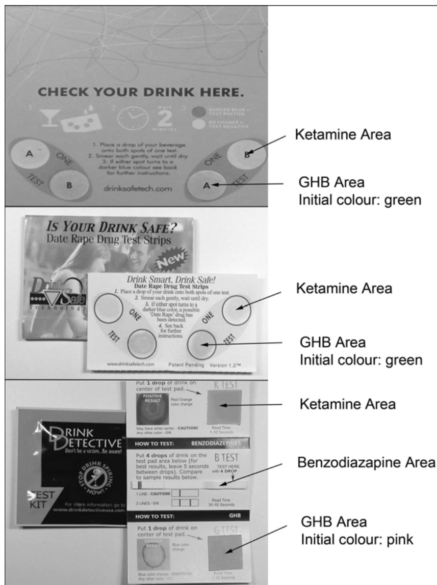
Figure 1. “DrinkSafe™” Coaster (top), “DrinkSafe™” Card (middle) and “Drink Detective™” Test Kit (bottom).
